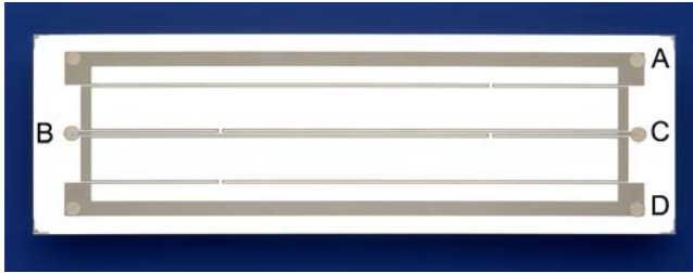
Fig. 1. Top view of the transient hot bridge sensor layout. Each of the four tandem-strips is 100 mm in length and 2 mm in width. Solder pads A, B, C, D: A-D, current source; B-C, DVM; (see Fig. 2) .
